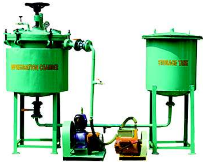
Vacuum Impregnation Plant
